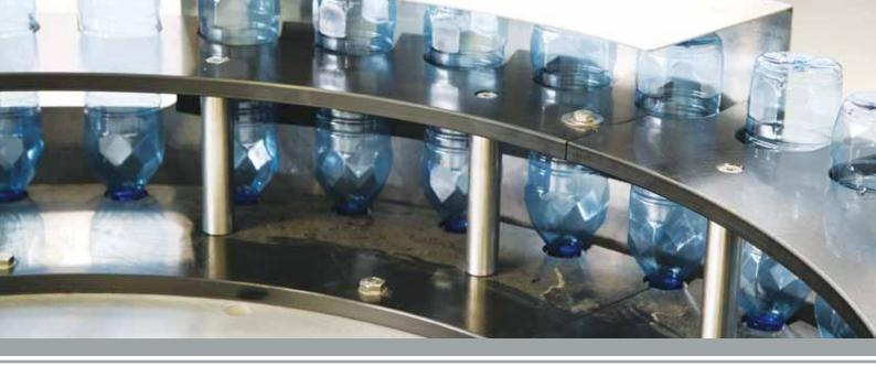
Filtec Automation offer a **Semi Automatic Bottle Rinser** to rinse bottles with water or ozonated water. Bottles are hand loaded into the rinser pockets in the star wheel as it rotates. A pump supplies rinse water under pressure to the rinse nozzles to rinse the inside of the bottles. The bottles then drain before being ejected to an external bin.
